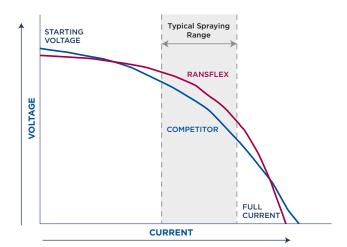
In the Typical Spraying Range, the RansFlex produces and maintains higher kV which results in better transfer efficiency and less overspray when using the direct charge applicator.
