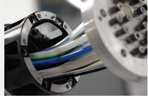
Color coded tubing bundle for easy change-outs and operational efficiency.
