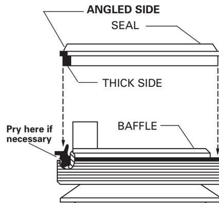
4. Assemble seal to baffle with angled side up as shown in diagram. **NOTE:** The seal should be a tight fit on the baffle. If it is a loose fit on the baffle, assure that it is assembled with the angled side up.
