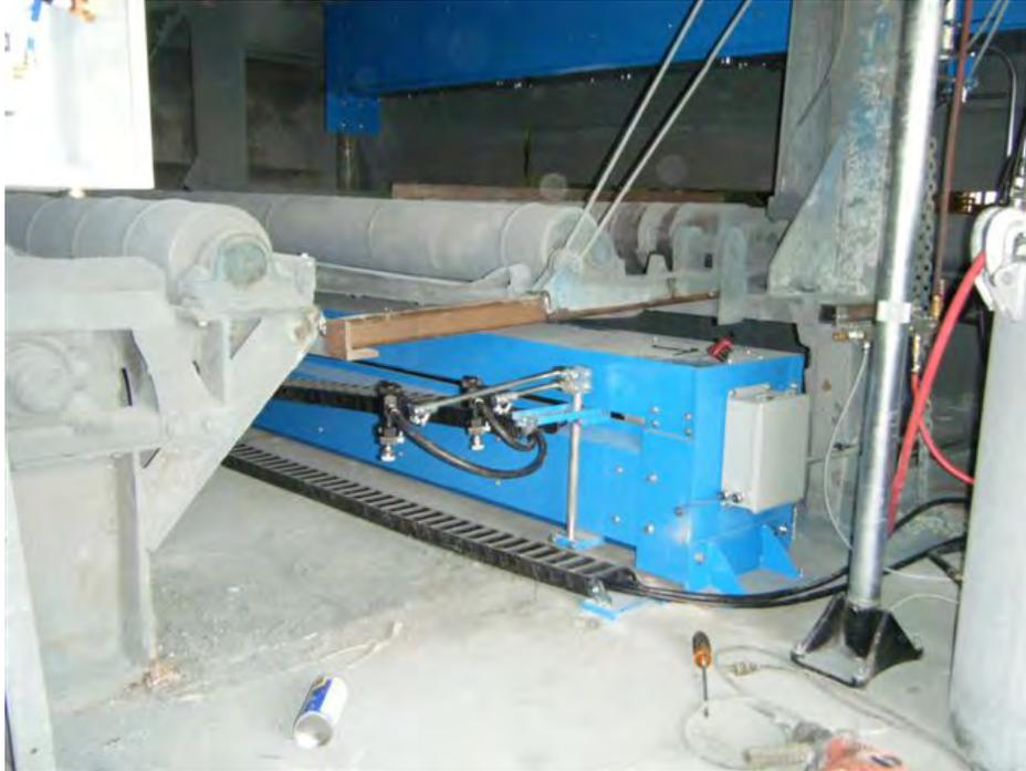
Sensor Array to determine Sheet Steel Size
